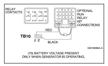
Figure 6-28 Run Relay Connections
